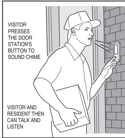
Figure 13. Door Station Operation
