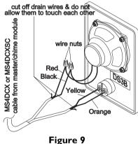
each door station location, strip approximately 4 inches of jacket from wire and separate colored conductors from one another. Strip 1/2 inch of insulation from each conductor as shown in figure 9. Cut each shield drain wire jacket to prevent them from touching each other (MS4DCXSC only). and **Terminate** yellow
