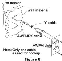
Connect the cable from the gang box to one of the 'Y' shipped with AWPM wall plate as shown in figure 8. Use the labels provided to mark the two jacks used and the two that are not used. Connect one of the 'Y' cables to the plate as shown and mount the plate using the two screws provided.
