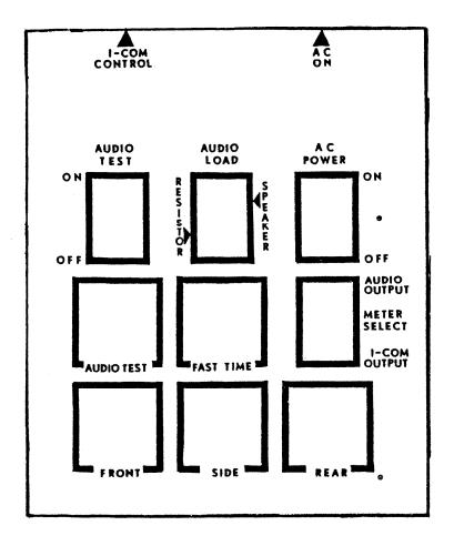
AC POWER: Switches 16 VAC to YELLOW and GREEN binding posts on and off. (Fixture on/off control by line cord)
